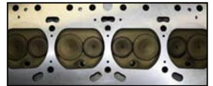
**Edelbrock heads with combustion chambers coated DMR-C-50012**
