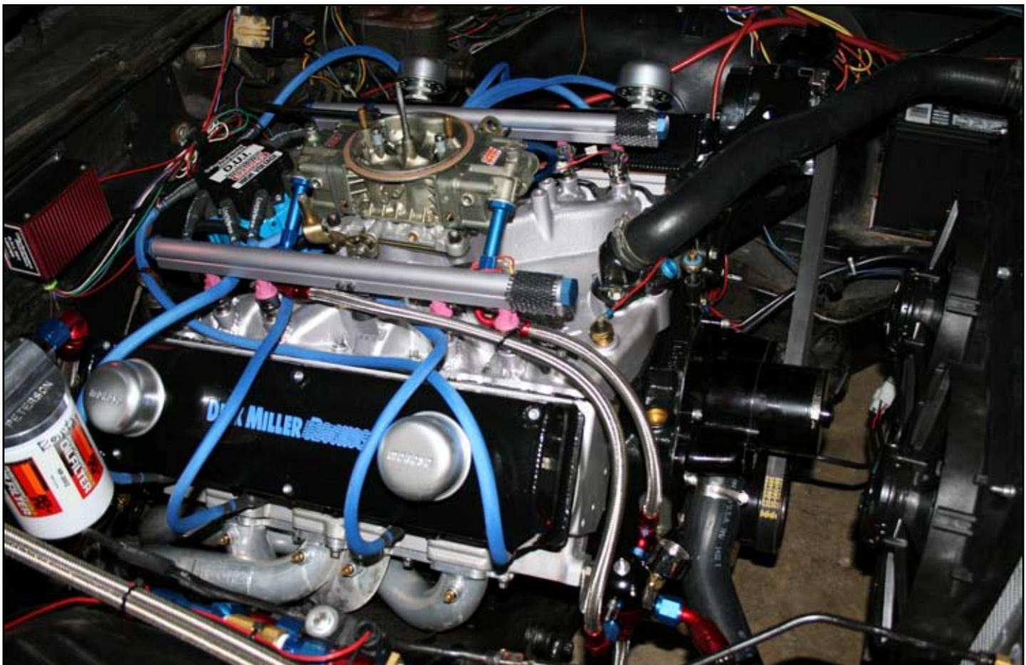
**CAR-4781-S4CTR 990 CFM modified carburetor. DUI-ITK-4270 distributor with external adjustment knob. DUI-9068 LIVEWIRES. DUI-380777 rev limiter. DMR-C-5005 protective coated intake. DMR-C-50051 protective coated heads. DMR-6813-RP headers Jet Hot ceramic coated. MAZ-WP-135S electric water pump. DMR-5065-2 serpentine pulley set. DMR-0100-E-P-B-4 sheet aluminum valve covers powder coated, engraved, with 4 breathers. These are all parts Dick runs on his 70 Cutlass.**
