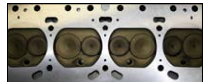
Edelbrock heads with combustion chambers coated DMR-C-50012
