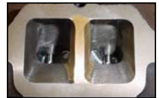
DMR-3003 ported head with center divider brased flush
