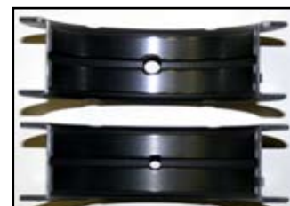
DRILLED VS. NOT DRILLED
